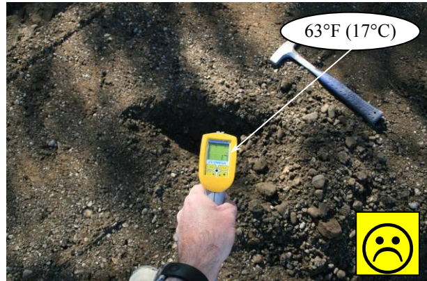
Figure 6.21: Recycled material (cold, poor dispersion).
