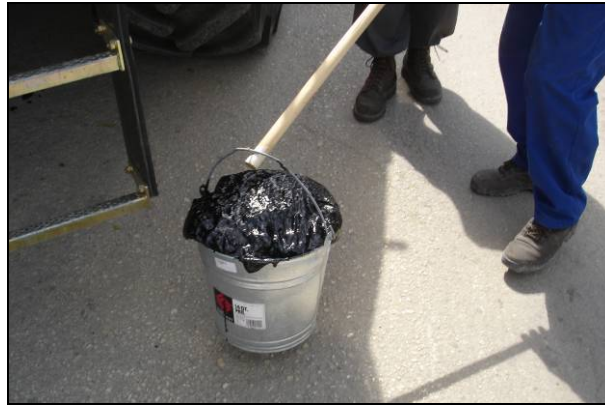
Figure 6.24: Checking expansion ratio and half-life.
