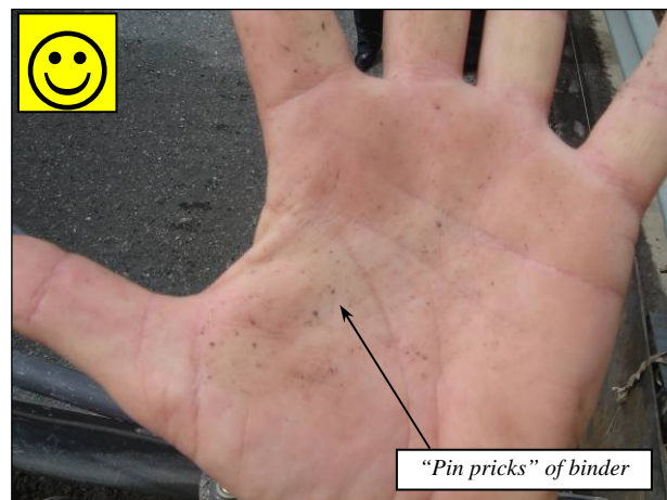
Figure 6.29: Moisture content checks (too dry and too wet).
